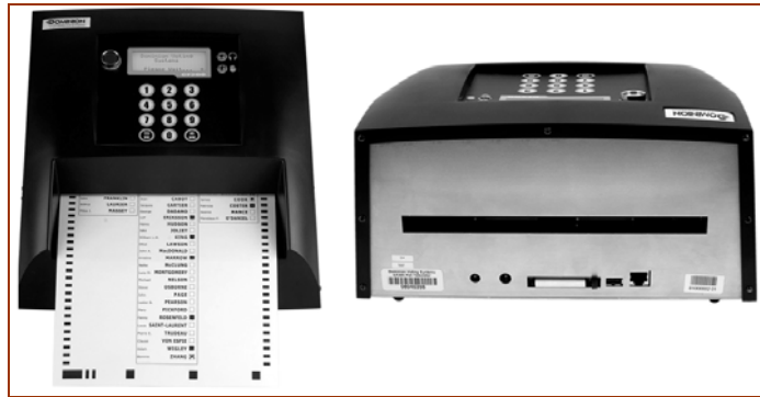
Figure 5: The CF200 electronic voting box in the form of optical poll-level tabulator.
